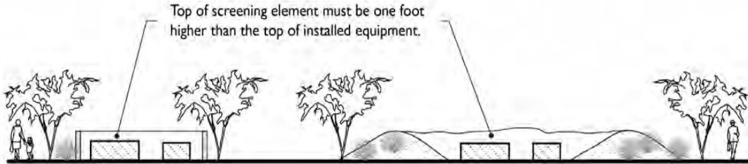
FIGURE 9311.7-B: SCREENING OF GROUND-MOUNTED EQUIPMENT
